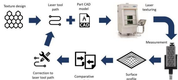
Figure 1. Close-loop manufacturing scheme being pursued in the SHARK project.
