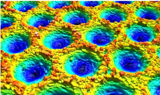
**Figure 4.** Laser textured friction disc (courtesy of MAN Energy Solutions). Lateral size of holes is in the order of 25 to 75  $\mu\text{m}$ . Depths range from 10 to 40  $\mu\text{m}$ . Obtained with a 50X Mirau 0.55 NA objective lens.
