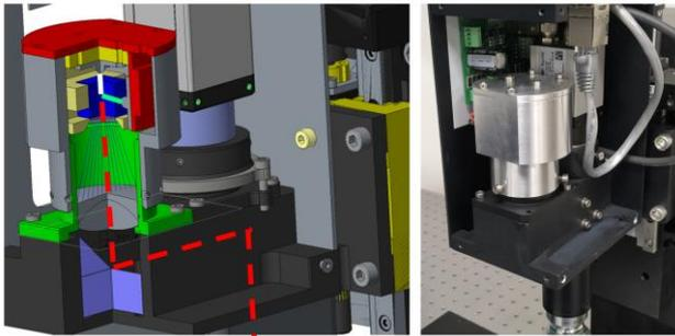
**Figure 3.** Dual LED arrangement: broadband (white) and monochromatic (green) light sources for high- accuracy and high-speed measurements: 3D cut model (left), prototype (right).
