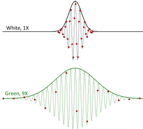
**Figure 2.** White and Green LED correlograms. In red, acquisition points for a single pixel, separated between them by  $\lambda/8$  multiplied by the speed factor: 1X (top) and 9X (bottom).
