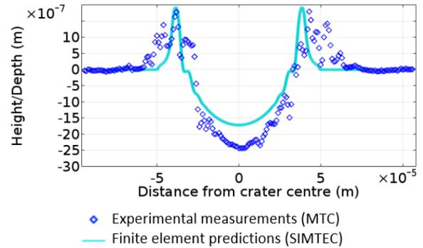
**Figure 7:** Experimental measurements from MTC (diamonds) and thermo-hydraulic FE model prediction (full line) of the crater profile from sample no. 4.
