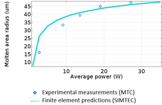
**Figure 4:** Molten area radius evolution with average power.
